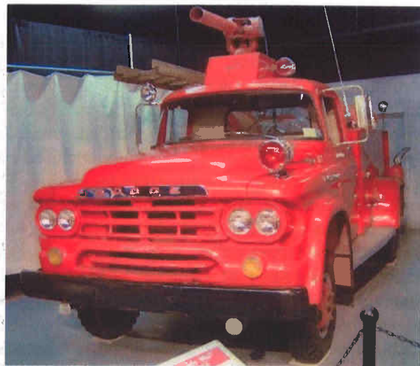
Mounted on a 1959 Dodge 4x4 chassis, Mahlon Irish's all-original American LaFrance "Little Mo" crash truck originally served in upstate Massena, N.Y. The formidable-looking cannon could pump water or foam while the vehicle was on the move.
